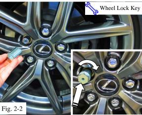
(b) Take the key supplied in the wheel lock set. Place it on top of the wheel lock and turn until the patterns engage. (Fig. 2-2)
